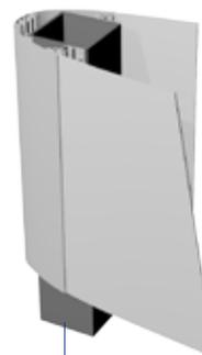
Aluminium or steel profile 80 x 80 x 4mm
